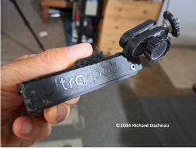
The "UltraPod"-I think they were made by "Pedco", but I've had these for a long time-had the strap torn off, and some of the vinyl feet lost. This allowed it to fit snugly into the top of the pole without any modifications.
