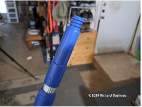
I bought an inexpensive paint roller handle to use for my camera base. I removed the frame from the handle, then cut a ¼-20 threaded rod to length (I didn't measure exactly, just assembled and cut as needed). Inside the handle, the rod is secured by a ¼-20 bushing, while outside, it is secured by two regular ¼-20 nuts. I've considered using at least one "nylock" style nut but haven't used one yet. I left threads exposed outside of the nuts.
