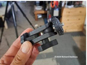
I mounted a jointed camera mount to the threaded rod. Then I threaded the new camera base assembly to the extension rod. The ¼ inch threads on that accept the mount for the GoPro. As shown, the mount will allow the GoPro to be adjusted to very many angles.
