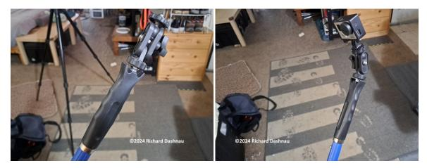
If necessary, I could drill and tap the altered handle assembly to accept a grub screw to prevent the handle from unscrewing from the extender. At this time, I don't think it will be needed. I have field-tested the second prototype. The images below show the appearance of the extended unit. As seen in the first image, there is a lot of flexing in the extended unit.
